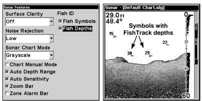
Sonar Features menu with Fish Symbols and Fish Depths highlighted (left). Sonar Page showing Fish symbols and FishTrack depths (right).
